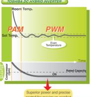
Toshiba has combined two technologies, creating the "DC Hybrid Inverter" that automatically chooses the better of the two control methods based on the actual conditions at the time. This solution provides high capacity only and when it is necessary.
